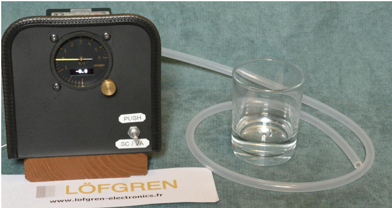
Now, position the open end of the instrument tubing just above the water (1). Plunge the open end of the tube to the bottom of the water glass and start the stopwatch at the same time(2). The variometer will show a rapid sink, needle moving away from zero. When the needle stops at it's maximum deflection (reverses direction, moving back to zero) stop the stopwatch.
